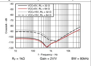
Figure 10. Crosstalk versus Frequency
