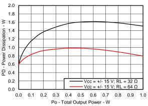
Figure 18. Power Dissipation versus Output Power
