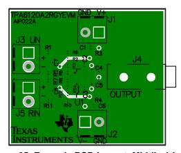
Figure 25. Example PCB Layout, Middle-1 Layer and Silkscreen, Top View
