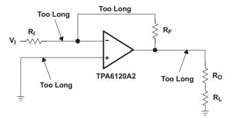
Figure 21. Layout That Can Cause Oscillation
