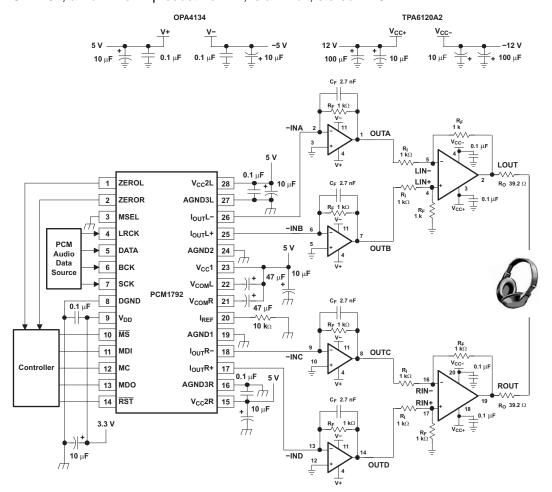
Figure 13. Typical Application Circuit
