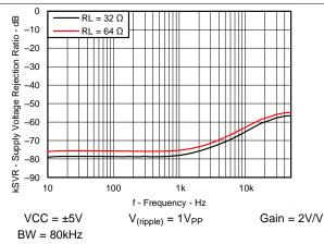
Figure 9. Supply Voltage rejection Ratio versus Frequency
