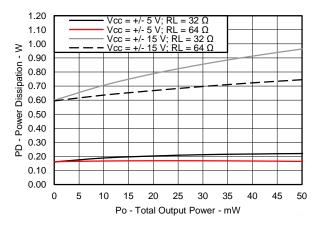
Figure 20. Power Dissipation versus Power Output - 50mW Scale
