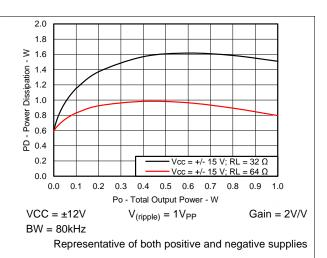
Figure 8. Power Dissipation versus Total Output Power
