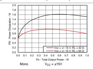
Figure 7. Power Dissipation versus Output Power
