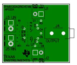
Figure 27. Example PCB Layout, Bottom Layer and Silkscreen, Top View
