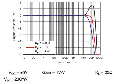
Figure 17. High Frequency Peaking for Oscillation and Instability
