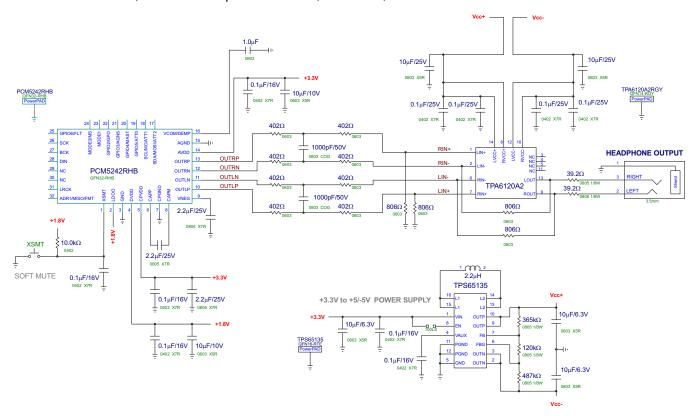
Figure 19. Typical Application Circuit
